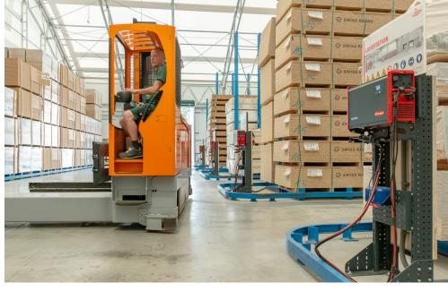
laboration with the customer the Fronius Perfect Charging team developed the ideal charging concept. Individually designed charging stations were planned, to suit the special requirements and dimensions of the heavy-duty forklifts. High reliability and particularly efficient and gentle charging of the powerful traction batteries were also a priority. The charging concept sustainably
