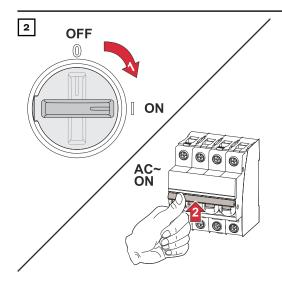
Set the DC disconnector to the "on" switch position. Turn on the automatic circuit breaker.
