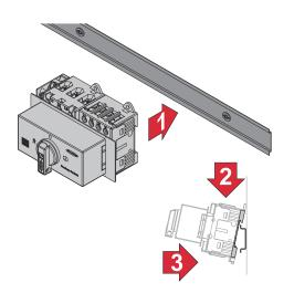
The Fronius Backup Switch can be mounted on a 35 mm DIN rail.
