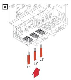
Plug the singles conductor (L1', L2', L3') coming from the backup power circuit into the terminals.
