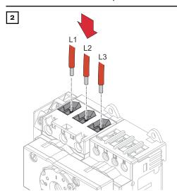
Plug the single conductors (L1, L2, L3) coming from the grid into the terminal.
