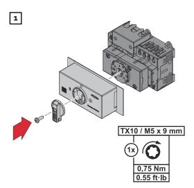
Reinstall the housing cover and the switch and secure with the screw.
