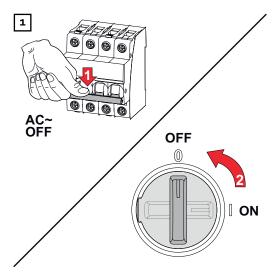
Turn off the automatic circuit breaker. Set the DC disconnector to the "off" (OFF) switch position.
