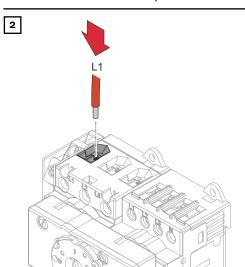
Plug the single conductor (L1) coming from the grid into the terminal.
