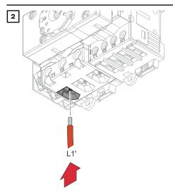
Plug the single conductor (L1') coming from the backup power circuit into the terminal.
