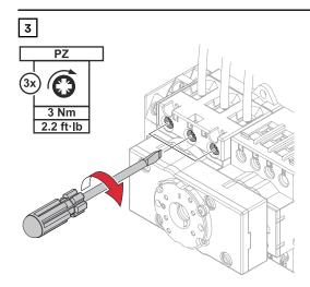
Tighten the single conductors (L1, L2, L3) in the terminals. For permissible connection screws and torques, see **Permitted connection screws** on page **19**.
