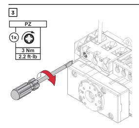
Tighten the single conductor (L1) in the terminal. For permissible connection screws and torques, see **Permitted connection screws** on page **19**. Connecting load 1-pin in the backup power circuit to the Backup Switch
