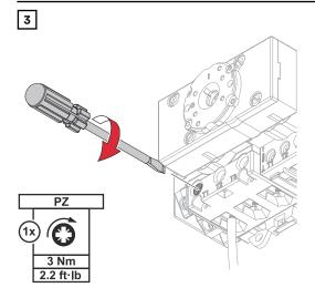
Tighten the single conductor (L1') in the terminal. For permissible connection screws and torques, see **Permitted connection screws** on page **19**.
