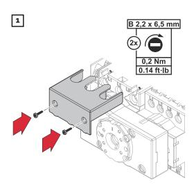
Mount a top protective cover on the load disconnector 63 A. Fit using the screws supplied with the delivery.
