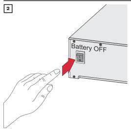
Switch off the battery connected to the inverter.
