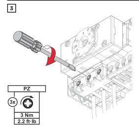
Tighten the single conductors (L1', L2', L3') in the terminals. For permissible connection screws and torques, see **Permitted connection screws** on page 19.
