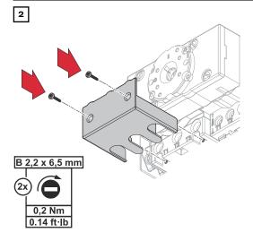
Mount a bottom protective cover on the load disconnector 63 A. Fit using the screws supplied with the delivery.
