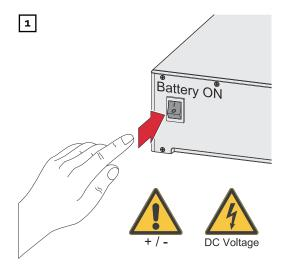
Switch on the battery connected to the inverter.
