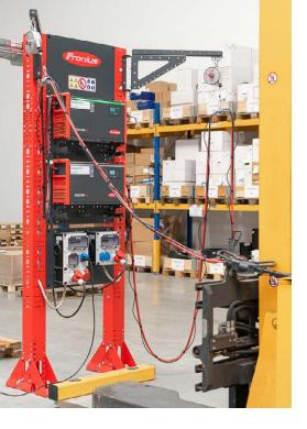
The LED strips on the battery chargers that are easy to see from a distance instantly show the employees at the Tornesch site which batteries are ready for use again.
