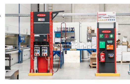
challenges together with the Fronius charging experts. In order to increase safety at work and minimize the fire load, the charging station had to positioned away from the storage racks. A free-standing, island solution was developed with Fronius to overcome these challenges. A special solution based on the Fronius charging module 2000 was designed with an overall height of 2.70 m to allow the power cables to be safely run above the modules via a cable bridge.
